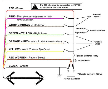
Note: The wires are shown above in order of Priority. Higher priority wires will override the patterns on any lower priority wires for the heads that are enabled.
